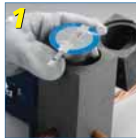
1 Insert CADWELD PLUS package into mould
